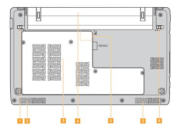
1 Battery latch - The manual battery latch is used to keep the battery pack secured in place.
